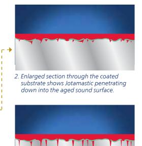
3. This section shows how Jotamastic, having penetrated deep into the substrate, converts from a liquid coating into a solid film.
