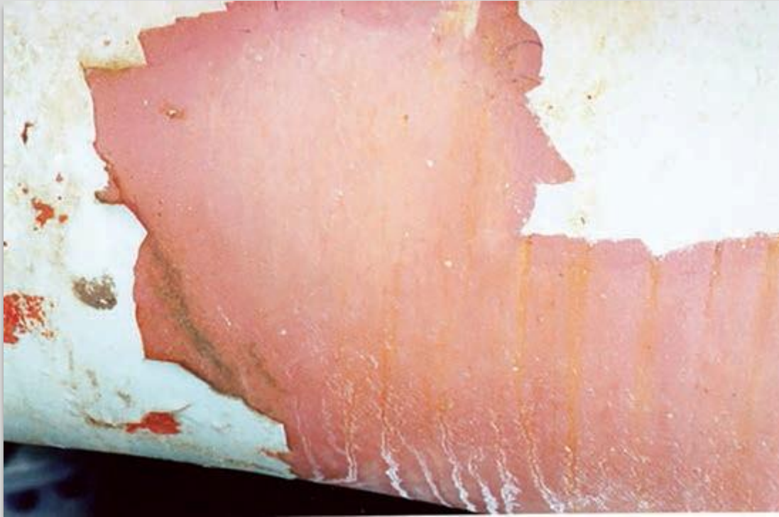
Fig. 24 Cracks that radiate from a point of impact.
