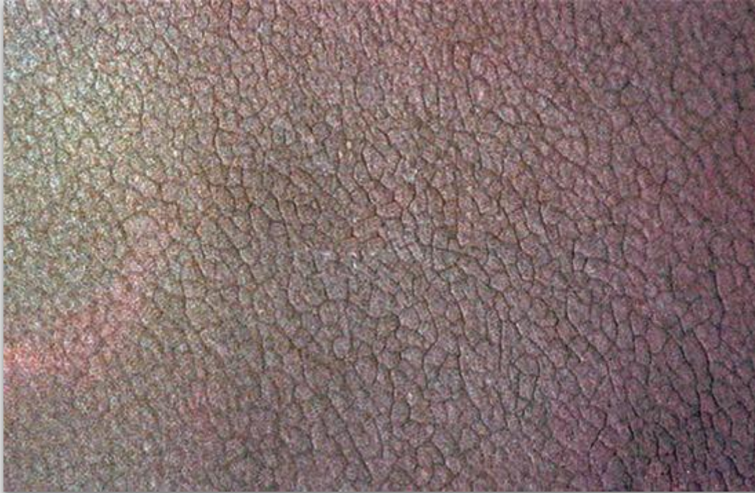
Fig. 25 The dried paint film has the appearance of a dried-out mud flat. The cracks appear as a network that can vary in size and amount.
