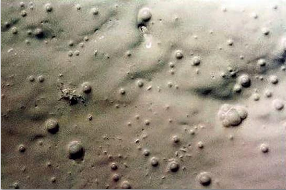
Fig.8 Bubbles within a paint film appear as small blisters. These may be intact or broken (leaving a crater). Can be found in excessively thick paint films, especially if spray applied, and also with roller application. This should not be confused with blistering.
