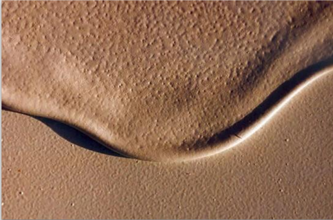
Fig. 34 Sags are caused by the downward movement of a coat of paint that appear soon after application and before setting, resulting in an uneven area with a thick lower edge. They are usually apparent on local areas of a vertical surface and, in severe situations, may be described as curtains.
