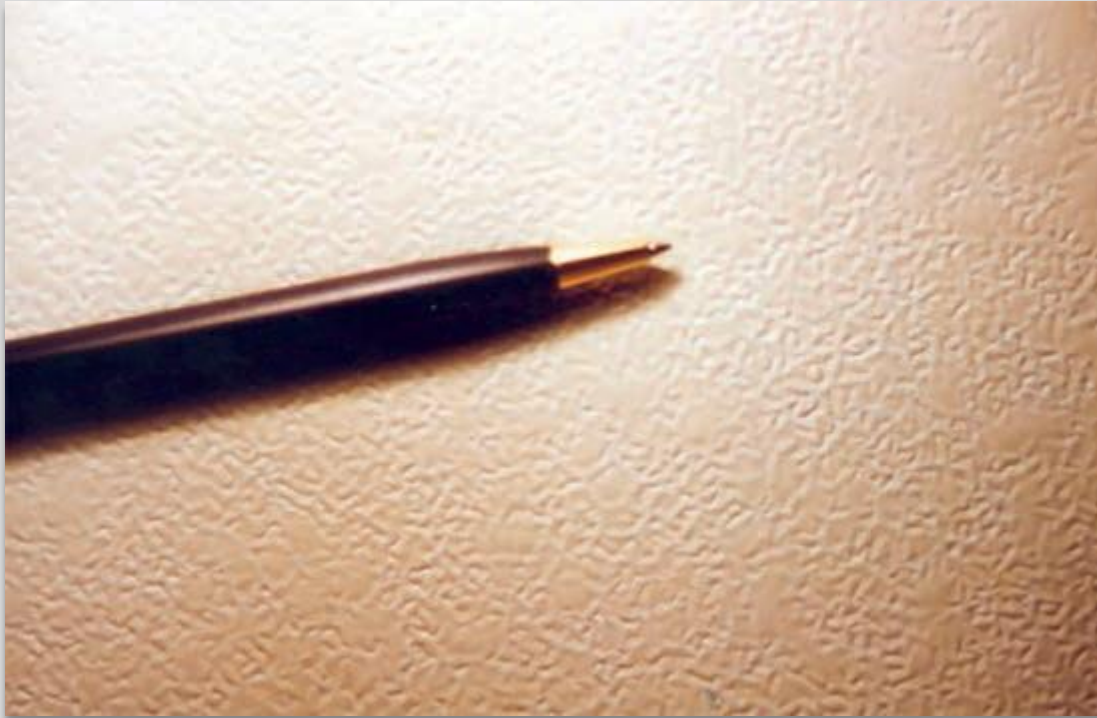
Fig. 26 A uniform, pock-marked appearance, in particular of a spray-applied coating, in which the surface of the paint film resembles the skin of an orange.
