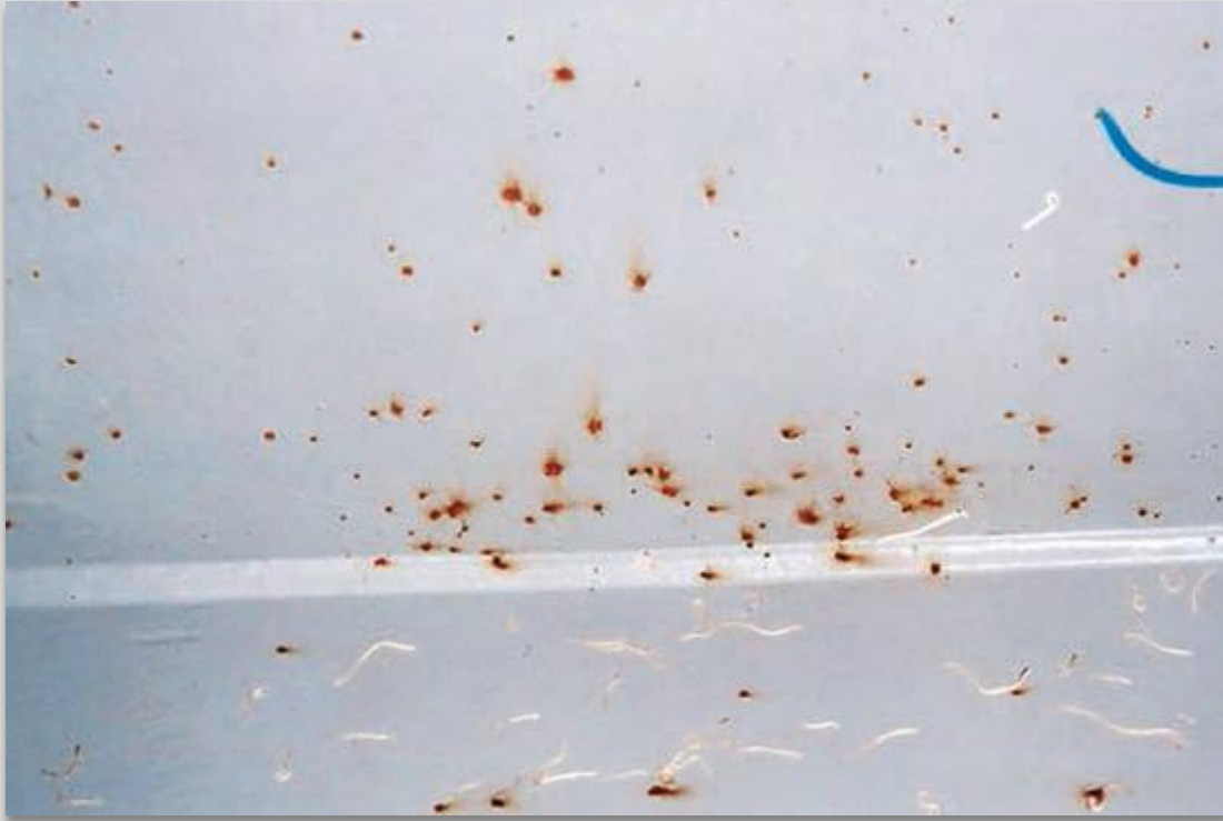
Fig. 32 Individual spots of rust that appear on a paint film and frequently start as localized spotting but rapidly increase in density.
