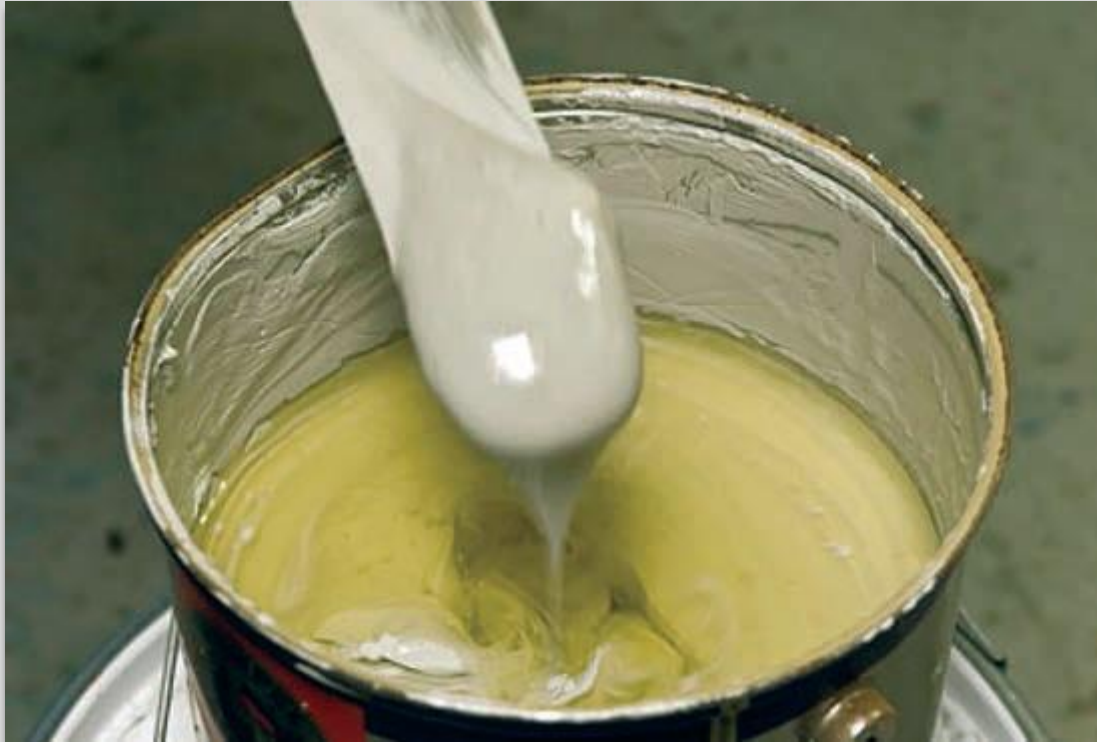
Fig. 35 The sedimentation of the solid constituents comprising pigments and extenders from the binder and solvent while standing in a container. Settlement that occurs after mixing and during application can result in different shades and performance in different areas.
