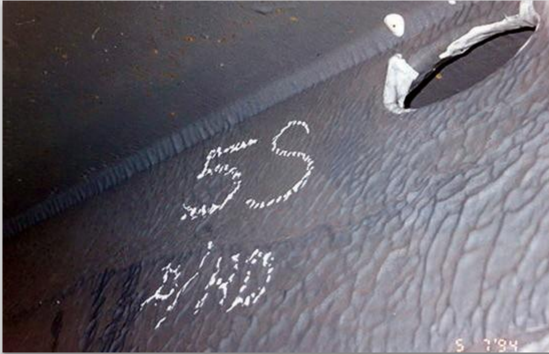
Fig. 29 A rippled effect on the surface of the paint.
