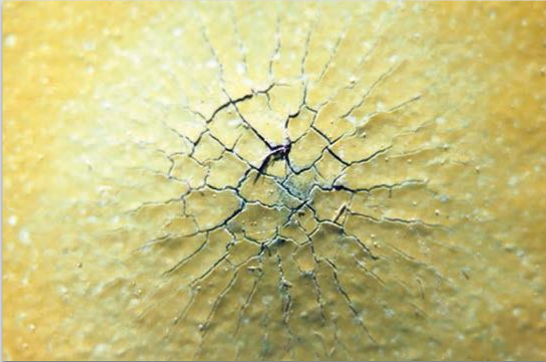
Fig. 23 Cracks that radiate from a point of impact.
