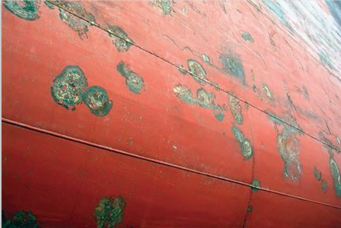
Fig. 9 Blistering and delamination of a coating system around bare steel areas and coating defects associated with cathodic protection on buried pipelines, immersed structures, and the hulls of ships.
