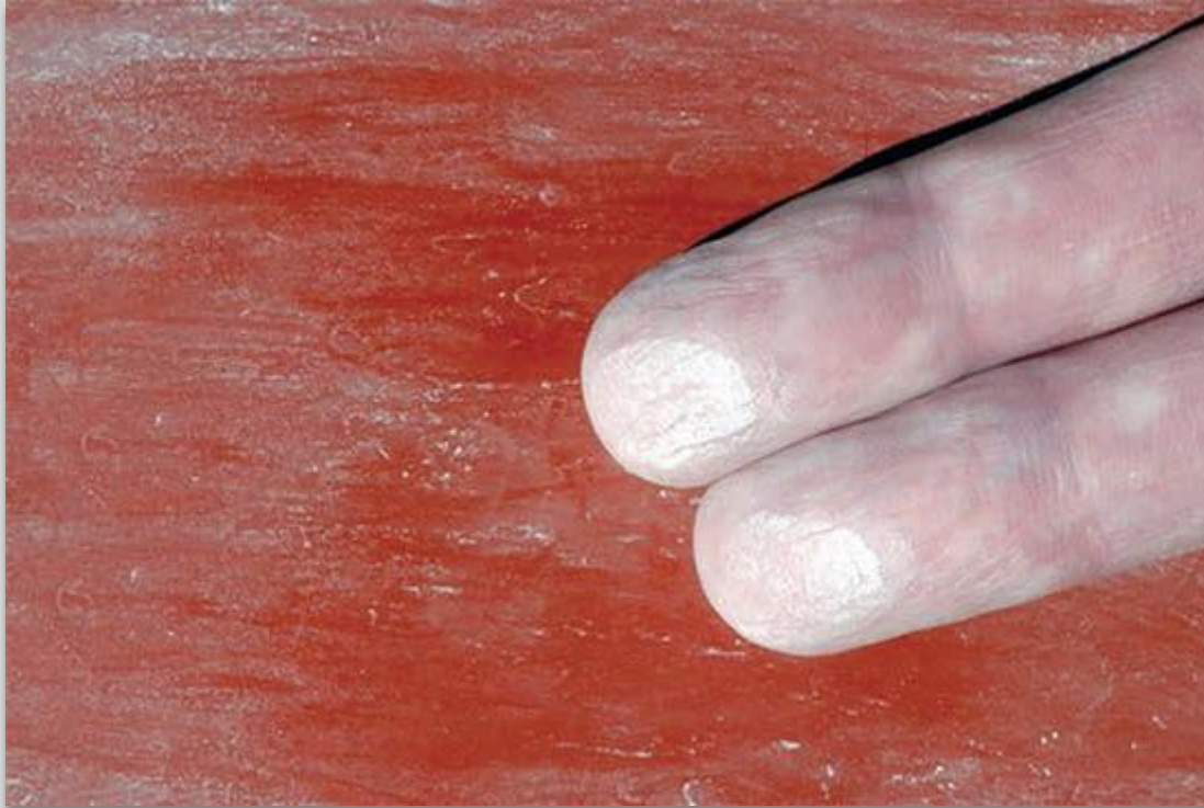
Fig. 10 A friable, powdery layer on the surface of a paint film. A change of color or fading is also seen. Chalking rates vary with pigment concentration and choice of binder. Chalking is a known characteristic of certain paints, for example, epoxy paints.
