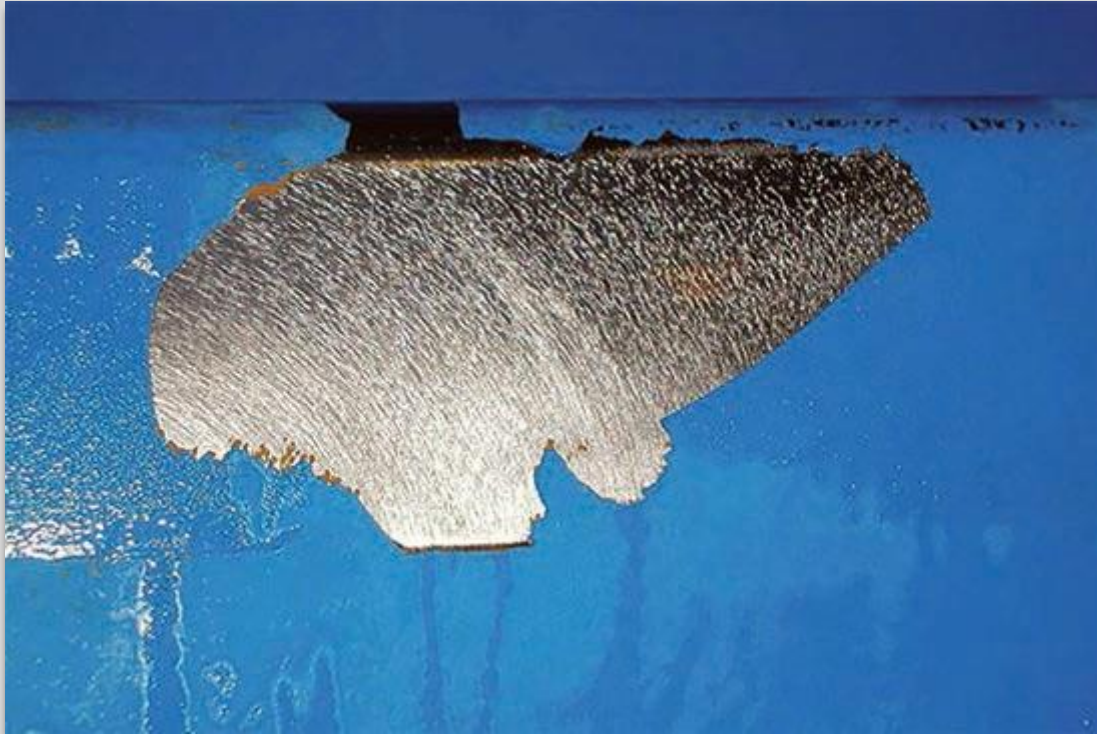
Fig.2 Paint fails to adhere to substrate or underlying coats of paint.
