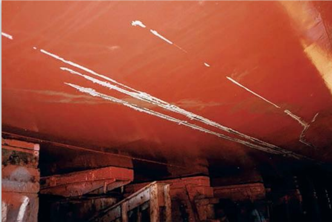
Fig. 1 The mechanical action of rubbing, scraping, scratching, gouging, or erosion.
