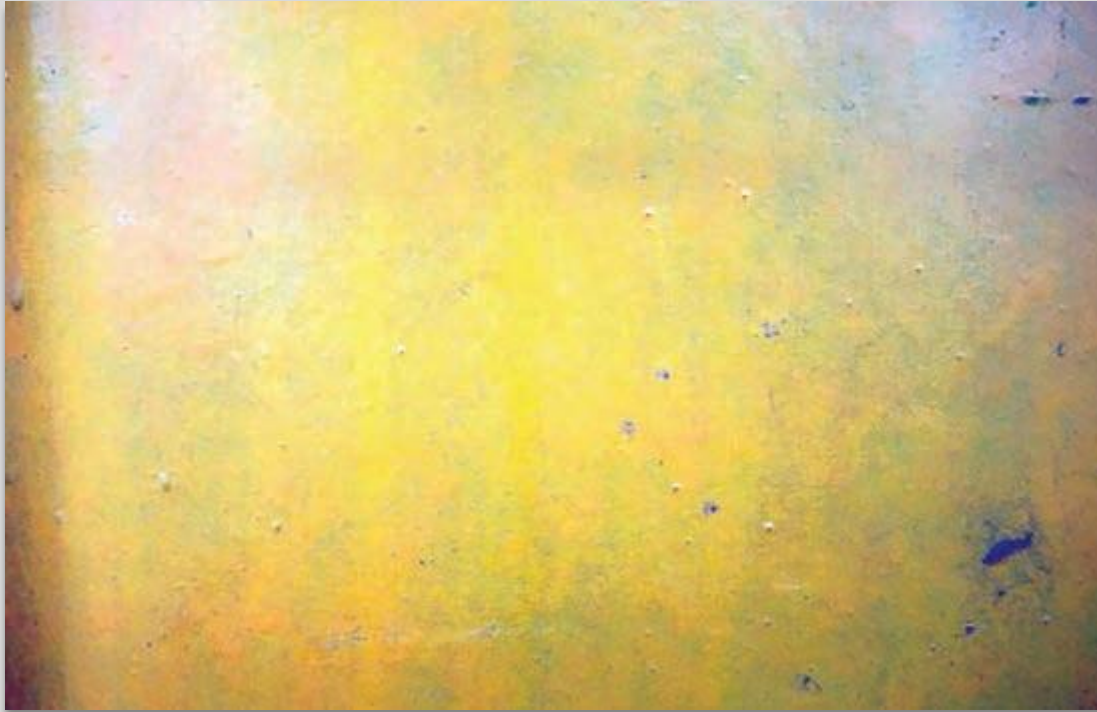
Fig. 21 The underlying surface is visible through the paint film due to inadequate hiding power of the coating material. This is sometimes called grinning-through. Often seen where dark colors are overcoated with lighter colors.
