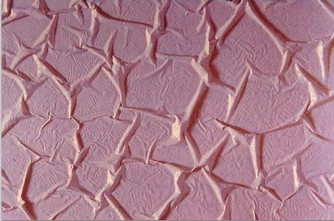
Fig. 42 The development of wrinkles in the paint film during drying.
