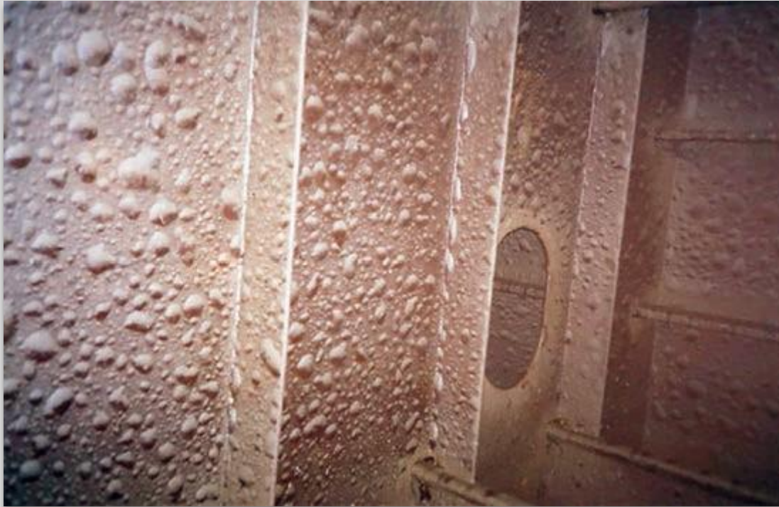
Fig. 5 Dome-shaped projections or blisters in the dry paint film through local loss of adhesion and lifting of the film from the underlying surface. Blisters may contain liquid, vapor, gas, or crystals.
