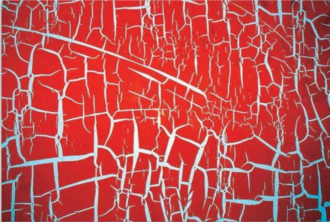
Fig. 3 Very large (macro) crazing/cracking that resembles the skin of an alligator or crocodile. Cracks may penetrate through to the undercoat or down to the substrate.
