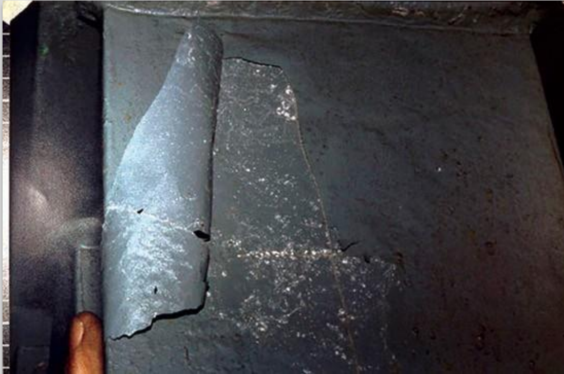
Fig. 27 Similar to flaking, although peeling tends to be associated with soft and pliable fresh coatings that can be pulled away from or spontaneously flake away from the substrate or from between coats, due to loss of adhesion.
