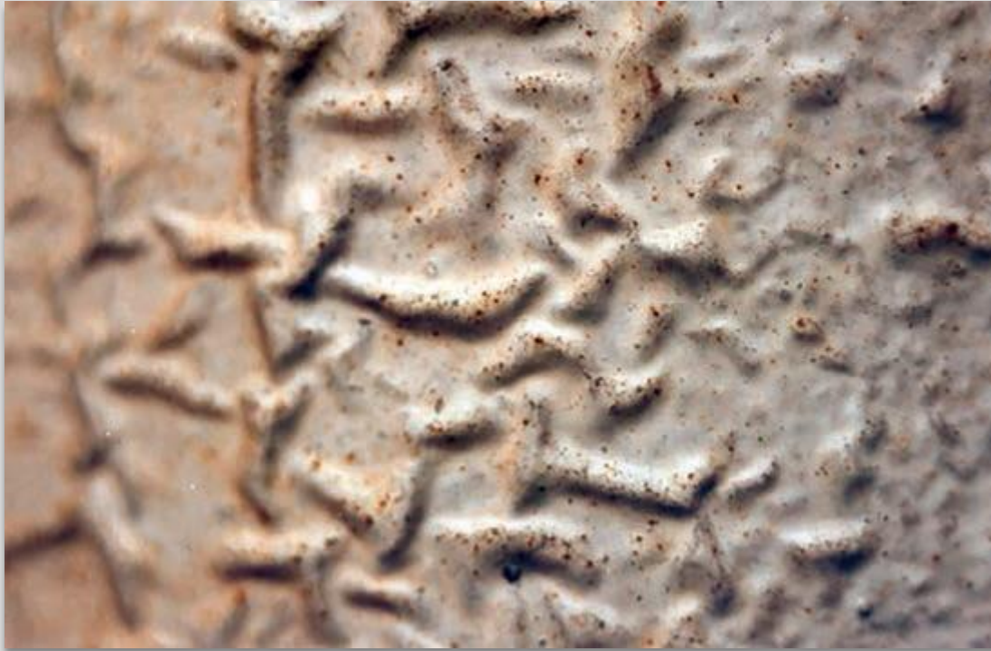
Fig. 37 Eruption of the surface of the paint film. Wrinkling and blistering, which lead to a weak surface and ultimate coating breakdown.
