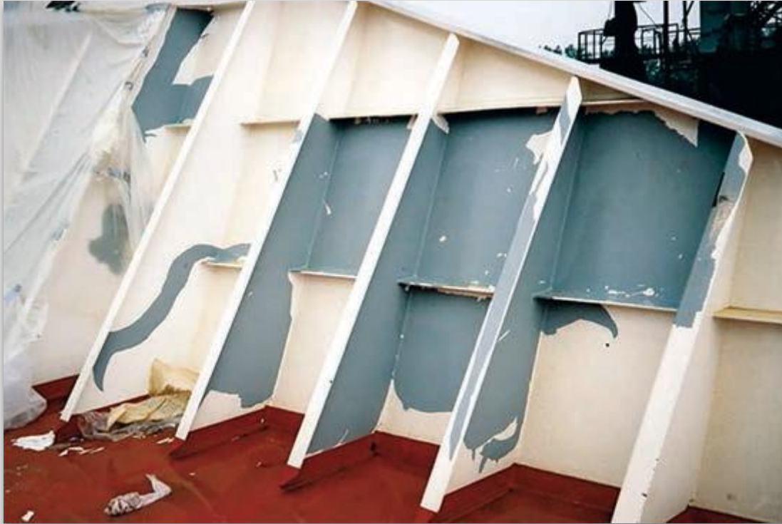
Fig. 18 Loss of adhesion between coats of paint.
