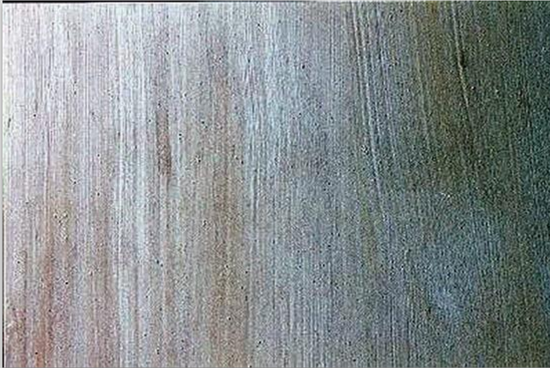
Fig. 4 Staining of a paint film by diffusion of a soluble colored substance from the underlying paint to give undesirable discoloration or staining. Often seen where bituminous- or tar-based products are overcoated with topcoats in which the tar or bitumen is soluble. Also occurs with emulsion paints.
